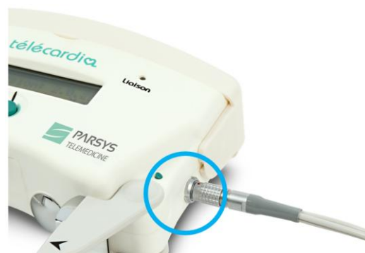
Peripheral cable connection The insertion mark, a red point on the cord, must be facing the device's top
