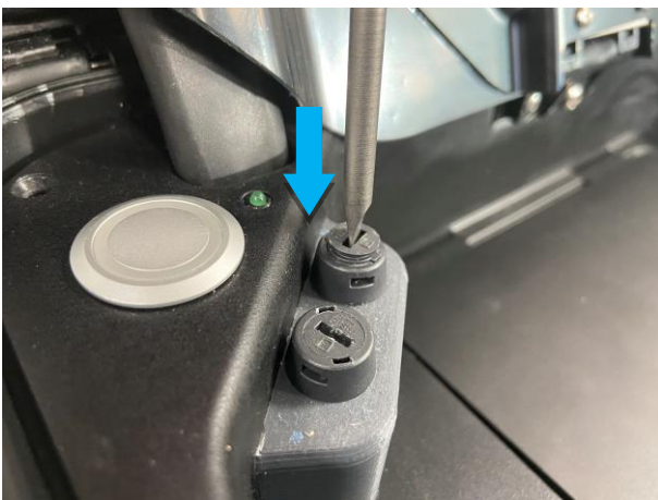
Reinsertion and press of the cap with its fuse
