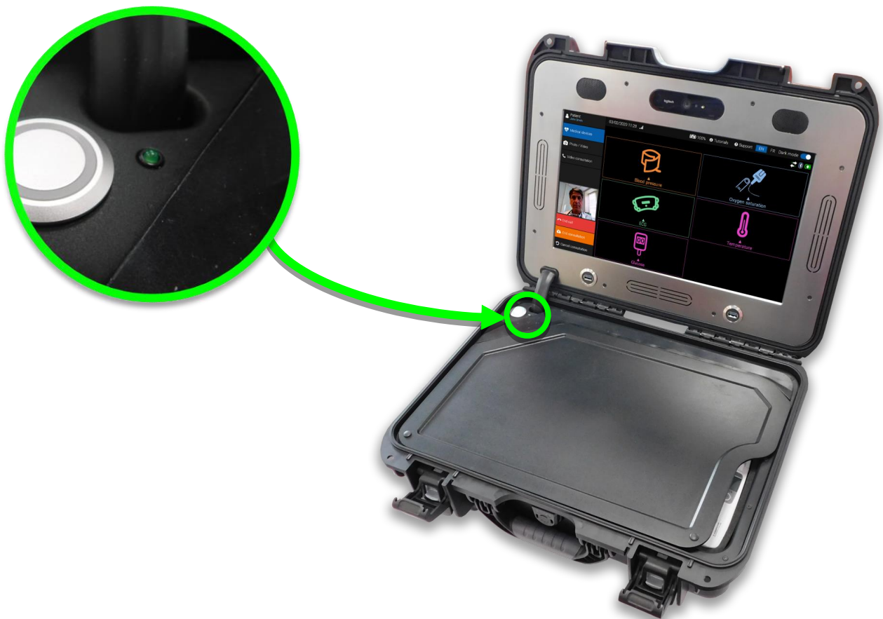
LED status Station battery position
