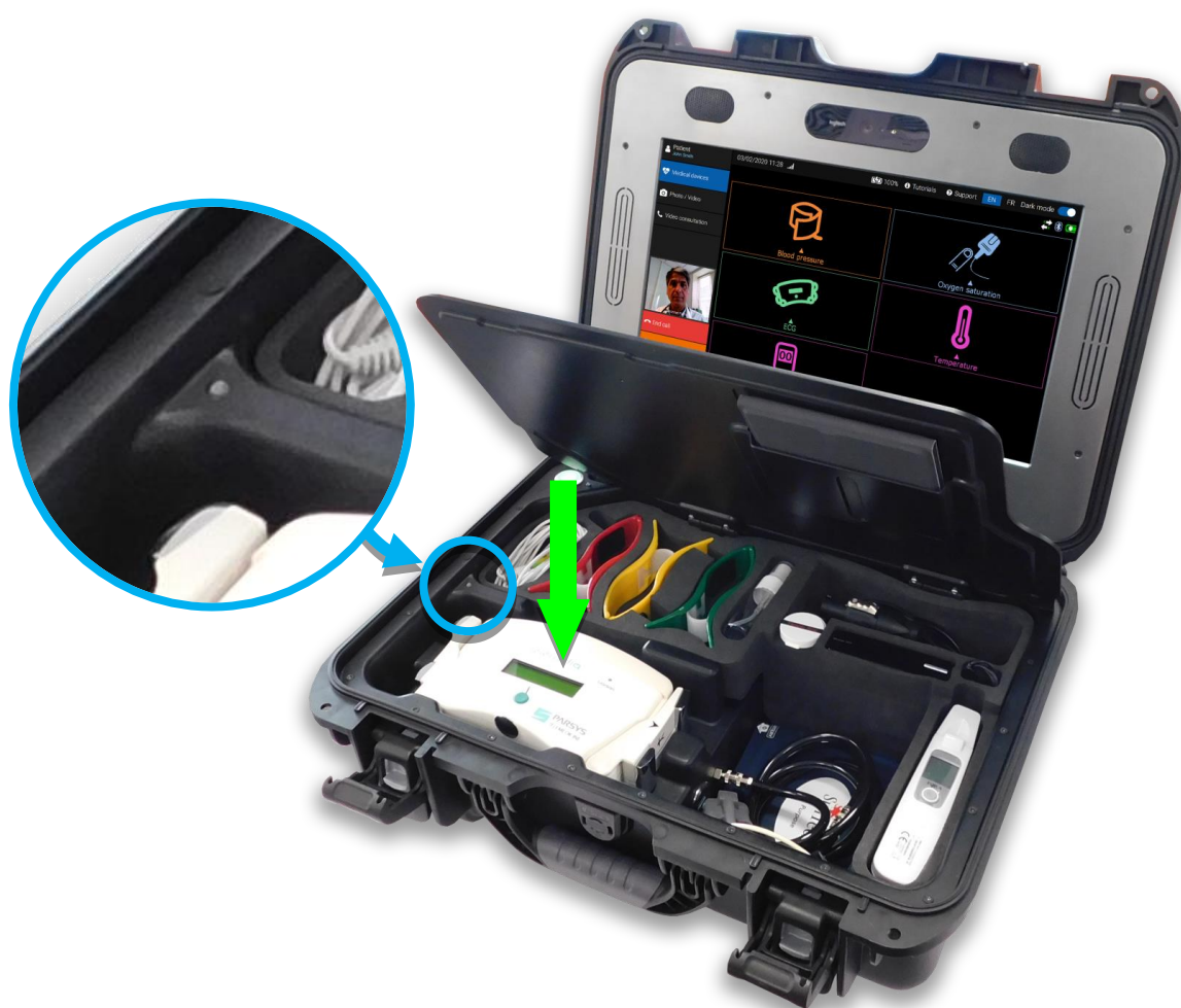
Insertion of Telecardia in its charging location and charging indicator position
