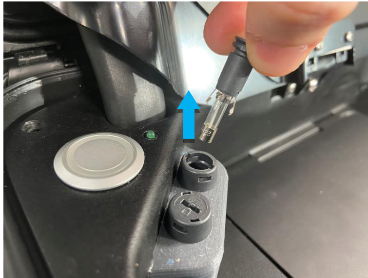
Removal of the cap retaining the fuse to be changed
